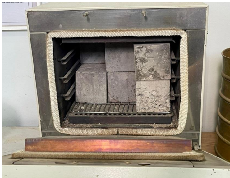
Fig 8.16 heating the cubes and crushing them on the testing machine
