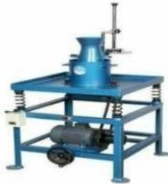
Fig 5 : VEE-BEE CONSISTOMETER TEST
