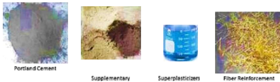
Figure 7.4: Main components of UHPC
