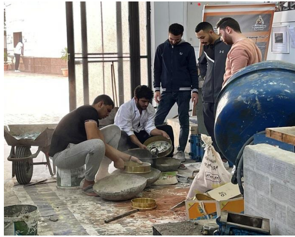
Fig 8.7 place the marble powder on sieve 4.75
