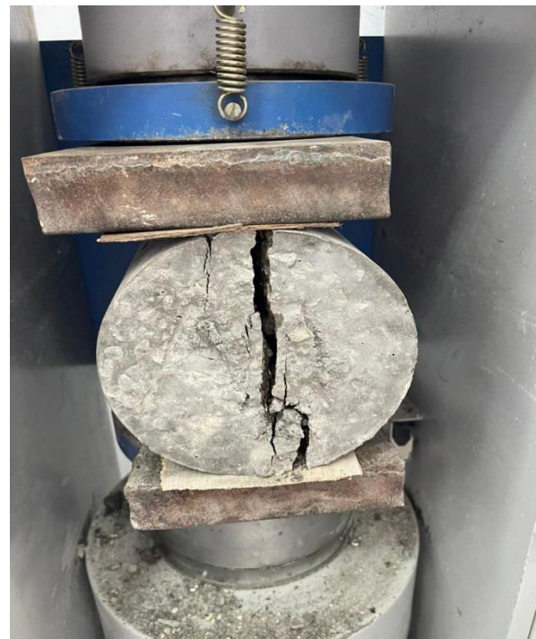
Fig 8.17 Brazilian tensile testing of concrete cylinders
