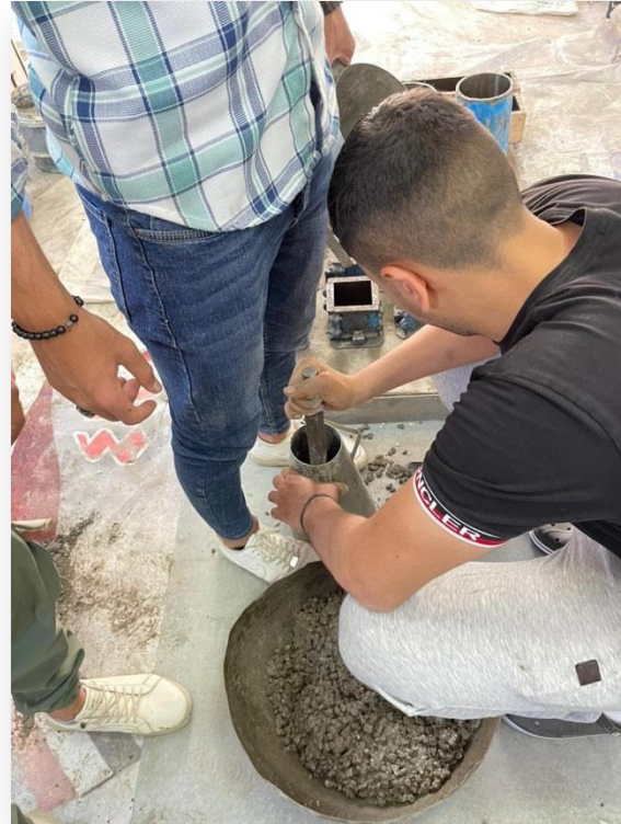
Fig8.3.2.1.2: Tamp the concrete into the cone
