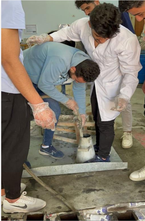
Fig8.3.2.1.2: Tamp the concrete into the cone
