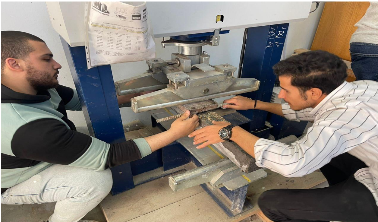
(e) Fig 8.18 Bending test for Beams
