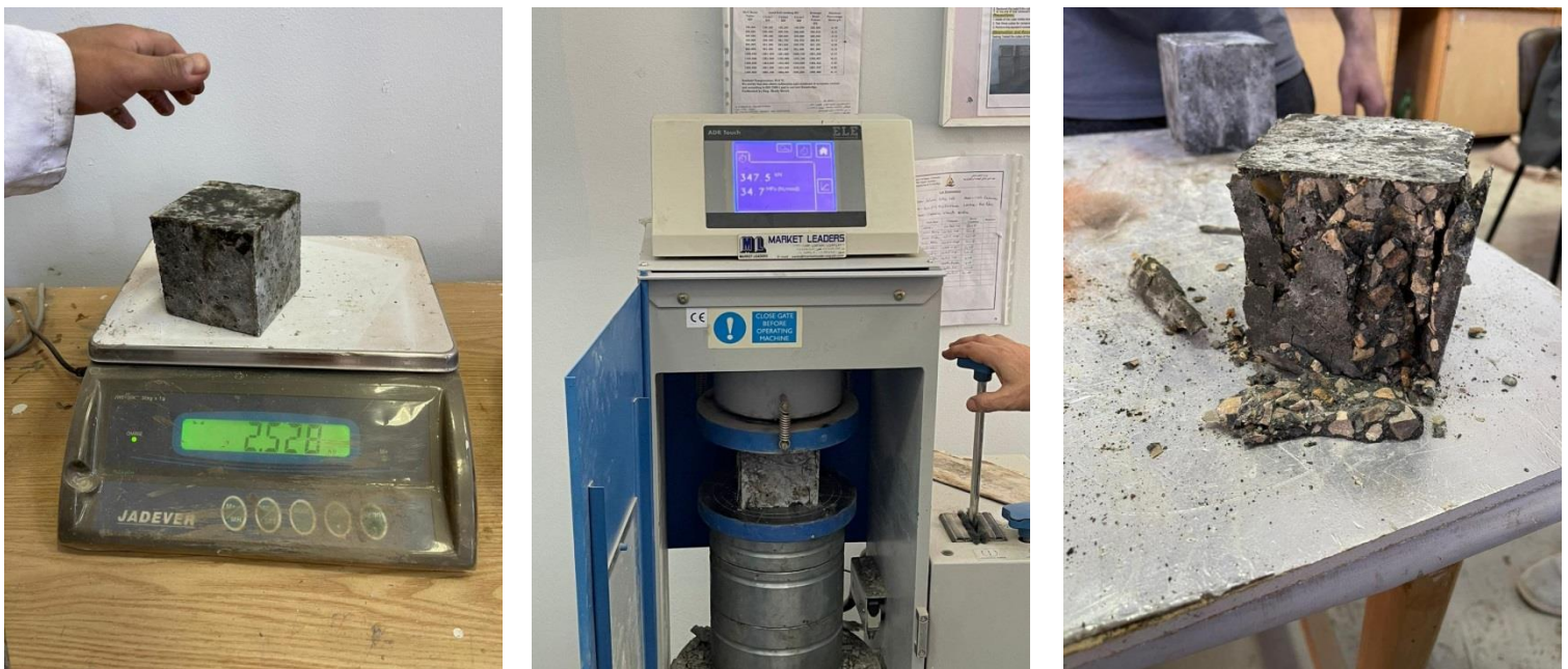
Fig 8.15 weighing and testing cubes on a pressure device
