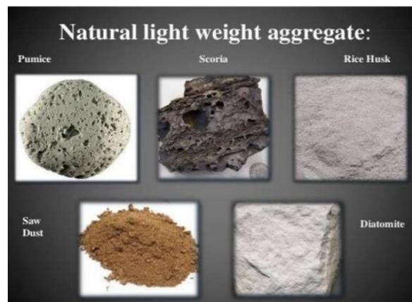
Fig-2 Natural lightweight aggregate: Pumice Scoria Rice Husk SawDust Diatomite
