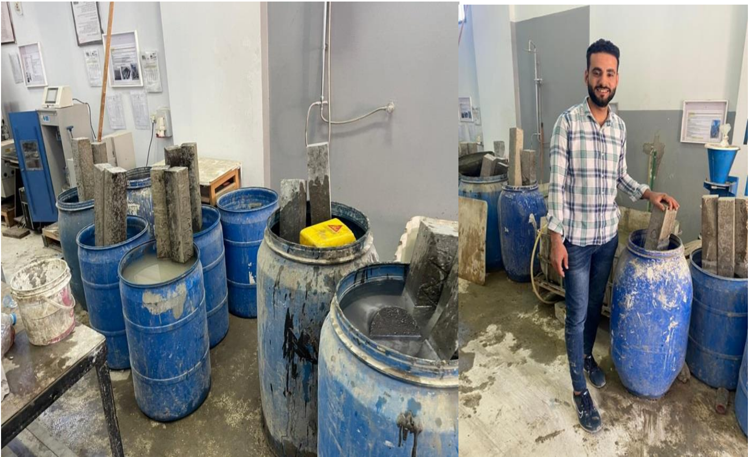
Fig 8.18 curing samples in water
